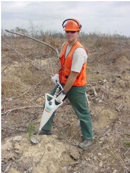
Figure 34. Jason Helvey with Kioritz soil injector.
