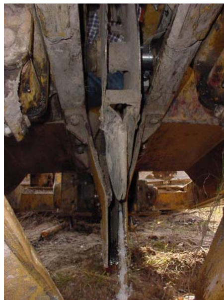
Figure 38. Dispensing fipronil solution from tubing in planter sleeve.
