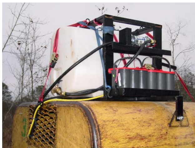
Figure 37. Injection system (tank, pump and battery power) fitted to top of machine planter.
