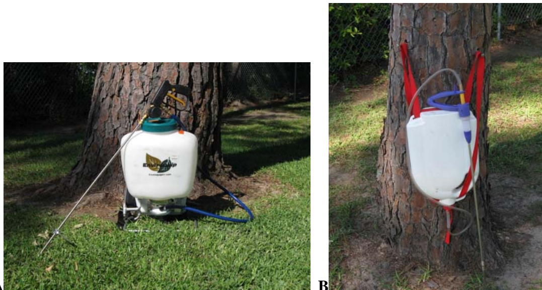
Figure 2. Soil injection systems: A) PTM™ Injection Probe and B) PTM™ Spot Gun
