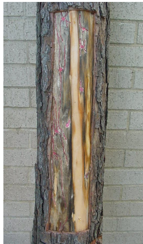
Fig 18. Fipronil-treated bolt with clear and colonized strips.
