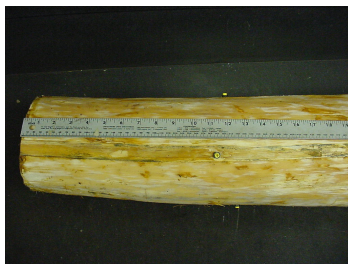
Figure 13. Lesion surrounding injection point on emamectin benzoate-treated bolt (May).
