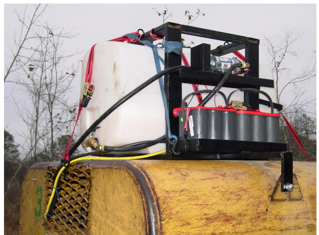
Figure 34. Injection system (tank, pump and battery power) fitted to top of machine planter.
