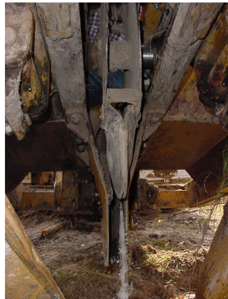
Figure 35. Dispensing fipronil solution from tubing in planter sleeve.
